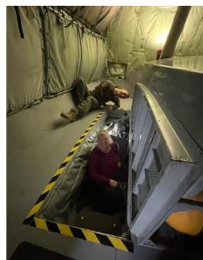
The boom operator lays on their belly to work the boom in the back of the aircraft.
